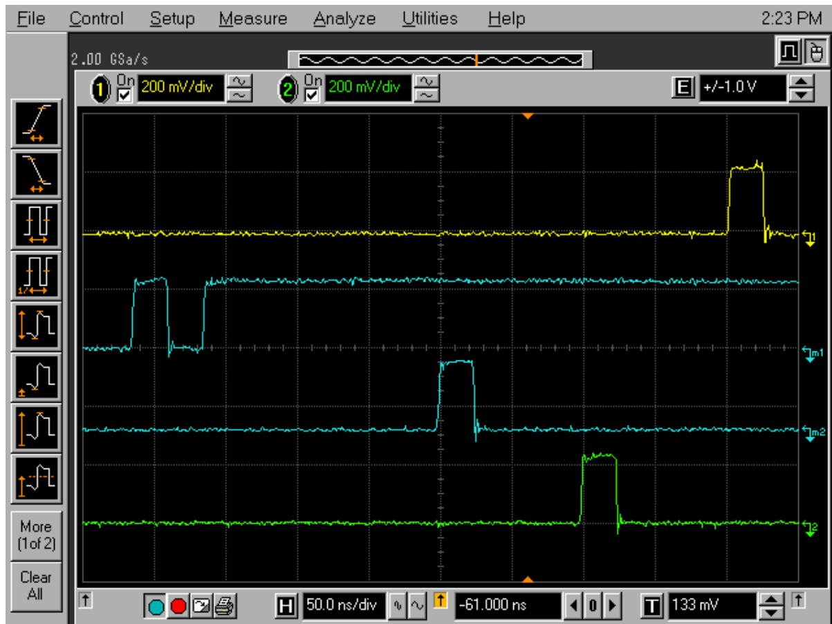
Figure 5.1 Prepulse to L0 delay at the TTCrx output for two different settings of the PP_TIME register: 3482 and 3486
